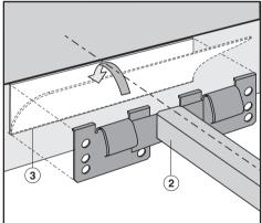
Position and secure the spring clamps ① and spacer bars ② using strong, double-sided adhesive tape ③.
